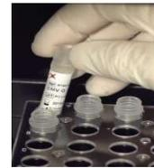
7. Load: PCR cassette, the ELITE InGenius SP RNA extraction cartridges, the ELITE InGenius DNase I and all the required consumables
