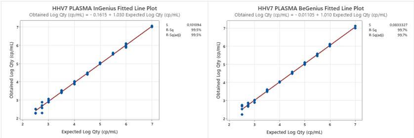
The results obtained by **ELITE InGenius** and **ELITE BeGenius** were analysed by orthogonal and linear regression in order to calculate the correlation between the methods. The results are summed up in the following figure.
