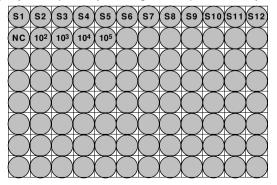
Legend: S1 - S12: Samples to be analysed; NC: Negative Control of amplification; 10<sup>2</sup>: 10<sup>2</sup> standard copies; 10<sup>3</sup>: 10<sup>3</sup> standard copies; 10<sup>4</sup>: 10<sup>4</sup> standard copies; 10<sup>5</sup> standard copies.
