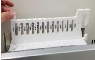
7. Load: Filter Tips, Extraction rack, and PCR rack
